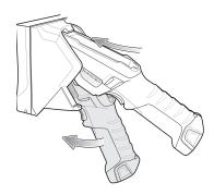
2. The TC8300 starts to charge automatically. The TC8300 charges in approximately four hours.
