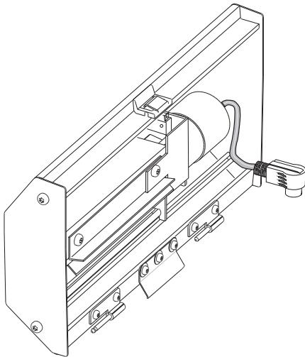
Cutter Installed PX4ie Printer
