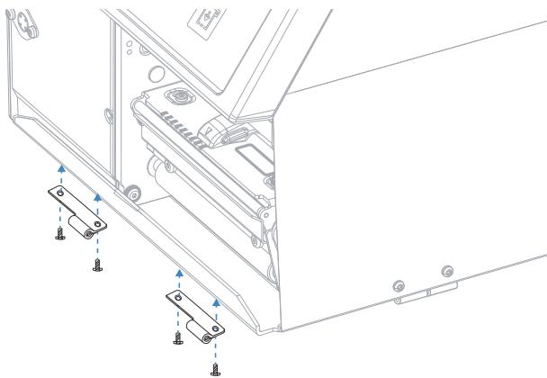
7. Fit the cutter unit to the vacant hinges. Make sure that the locking plate snaps into the groove of the right-hand hinge and that the angled plate at the bottom of the cutter is inserted under the printer's bottom plate.
