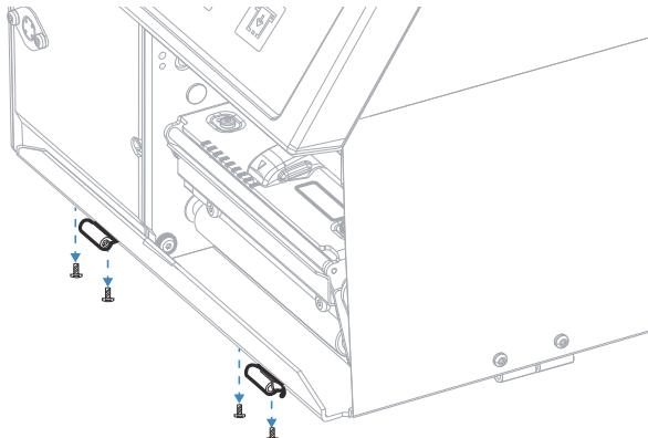
6. Replace the hinges with the new ones that came with the cutter unit using the same four #T10 Torx screw.
