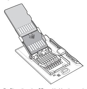
7. Close the microSD card holder door and slide the door to the Lock position.
