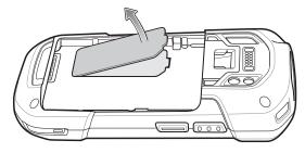
4. Slide the microSD card holder to the Open position.
