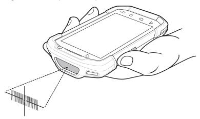
Press and hold the scan button.The red laser aiming pattern turns on to assist in aiming.
