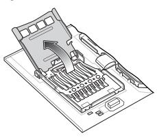
6. Insert the microSD card into the card holder door ensuring that the card slides into the holding tabs on each side of the door.
