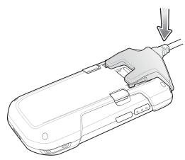
2. Rotate away from the device. The magnetics release the cable from the device.
