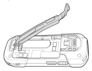
3. Insert the battery, bottom first, into the battery compartment in the back of the device.
