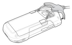
2. Rotate the cable down and press until it snaps into place. Magnetics hold the cable to the device.
