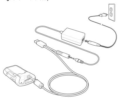
3. Connect to the power supply to an AC outlet.
