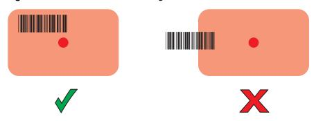
Figure 131 DS3608/DS3678 Pick List Mode with Multiple Barcodes in Aiming Pattern
