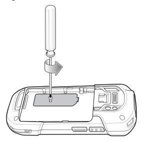
After re-installing the access cover, make sure to use a Microstix TD-54(3ULR-0) screwdriver to re-install the screw.
