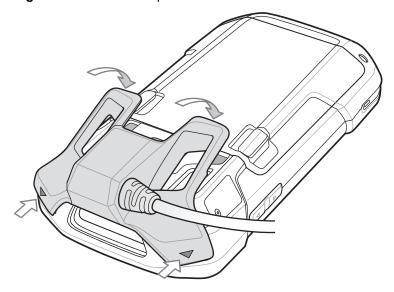
2. Rotate the Audio Adapter down and press down until it snaps into position.
