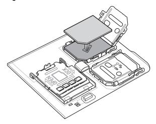
6. Close the SIM card holder door and slide to the lock position.
