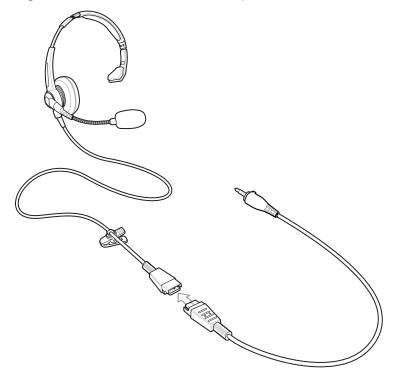
2. Connect the audio jack of the 3.5 mm Quick Disconnect Adapter Cable to the 3.5 mm Audio Adapter.
