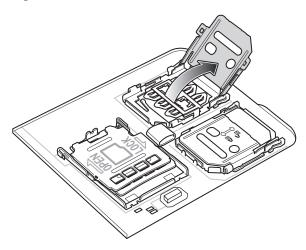
5. Place the nano SIM card into the card holder with contacts facing down.
