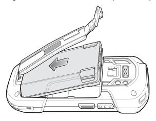
4. Press the battery down into the battery compartment until the battery release latches snap into place.
