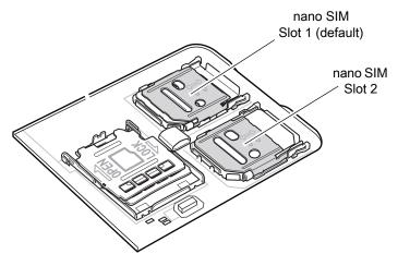
3. Slide the SIM card holder to the unlock position.
