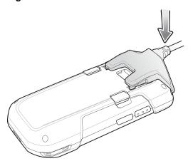
2. Rotate away from the device. The magnetics release the cable from the device.
