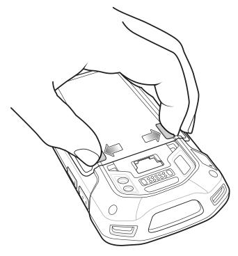
8. Lift the battery from the device.
